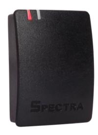
M20 Proximity reader is indigenously developed high performance reader to read Mifare read only cards. It provides a consistent read range of 4~5 cm in most of the conditions. The reader is particularly suited to access control applications. The same basic unit can be configured to most common output interface formats, including Wiegand, Magstripe and RS-232 serial ASCII.
